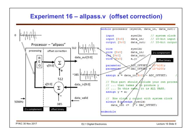
The ALL PASS module is slightly more complex than it may appear. Data\_in[9:0] is used to represent the analogue signal input (which is bipolar) as offset binary. There is an offset of around 385 if the input is connect to zero (no signal). The output data\_out[9:0] also has an offset. To get Vout = 0V, you need to send the binary number 512.
