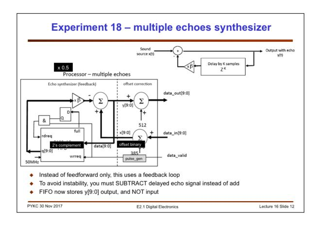
A slight modification create a mult-echo synthesizer. Here we put the delay element in a feedback path. Note that you MUST perform a subtract instead of an add, otherwise the system has positive feedback and will become unstable.
