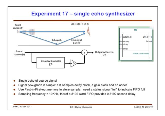
The final compulsory exercise is to create an echo synthesizer. The basic idea is simple: an echo is recreated when the listener receive the source signal via a direct path AND a delayed echo path as shown.
