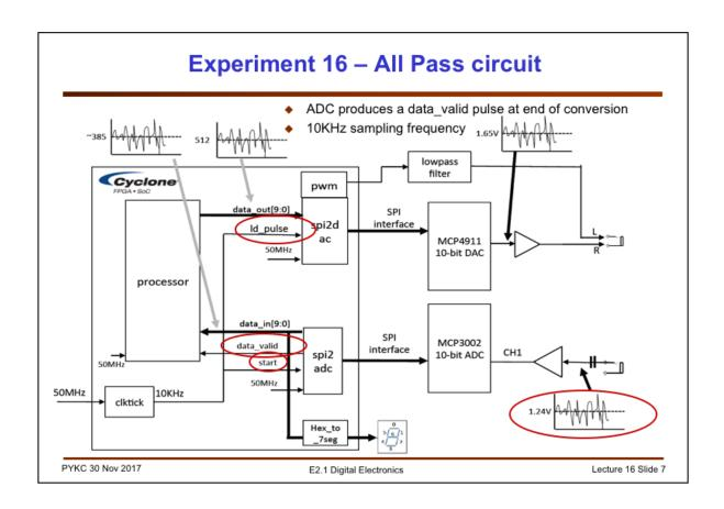
This is the block diagram of the basic framework used for Part 4 of VERI. The two main modules spi2dac.v and spi2adc.v provide interfacing to the DAC and ADC respectively. The control circuit is simple – a clock tick circuit generating a 10 KHz sampling clock The 7 segment displays can be used to monitor the ADC converted data.
