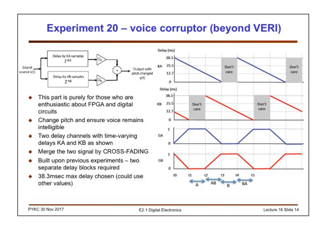
Finally, with minor modifications to the processing module, using TWO delay components and a variable gain (with time), it is possible to produce a pitch changer. There will not be enough time during the experiment for you to do this part. However, it may be a suitable Christmas project.
